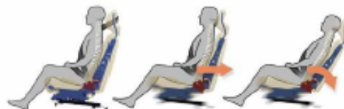
Autoliv/Volvo - WHIPS active whiplash protection
